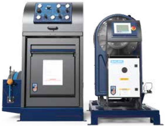
Fill station module showing optional hose reel
