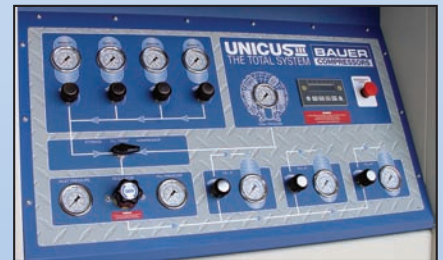
Hinged Cascade Fill Control Panel with Air Flow Schematic
