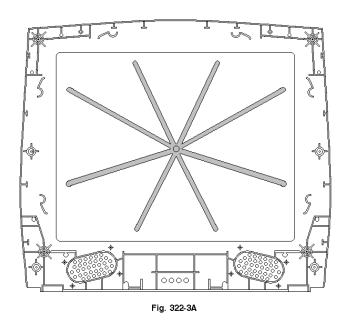
**FIGURE 322-3A** As is typical of many TV cabinet designs, this 25-inch cabinet front cover had a center cold sprue and eight runners supplying material to eight subgates.
