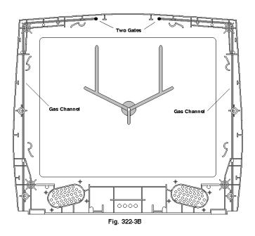
**FIGURE 322-3B** To convert to gas assist, six of the eight runners were welded, leaving two gates at the top of the cabinet. Gas channels were then cut in the core half of the tool.
